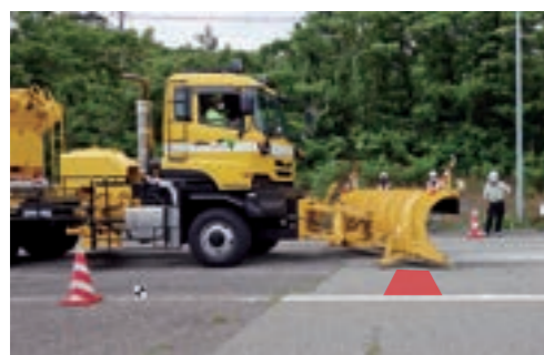
Testing automatic control (vertical movement) of a plow blade. A virtual bridge joint (red framed area in the figure) is set up in a test field to automatically test the plow blade moving up and down at the virtual joint.
