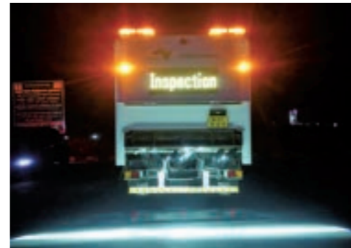
Road inspection by Road surface condition survey vehicle, E-NEXCO Eye
