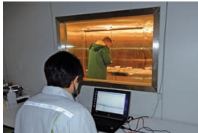
Testing solidification of antifreeze using a temperature and humidity test chamber
