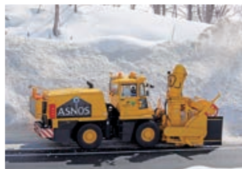
Test run of a snow blower with autonomous driving function
